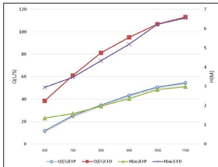
Figure 7 Comparison between experimental Q-H and CFD Q-H at various RPM
