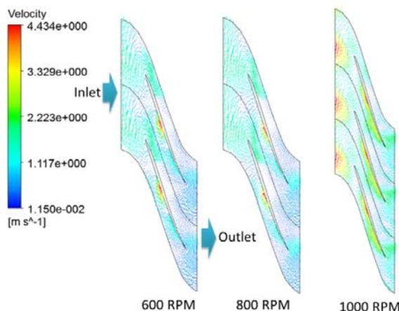
**Figure 9** flow structure Blade to Blade of various RPM
