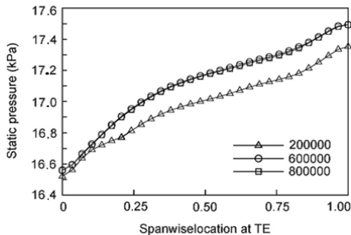
Figure 4 Grid dependency test results
