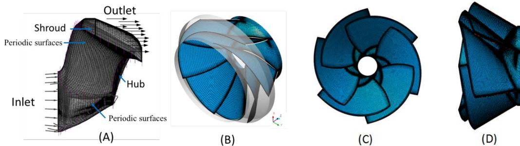
**Figure 2** Impeller flow simulation domain and structured grid
