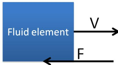
**Figure 8** Shear force acting on fluid element that moves with speed of V
