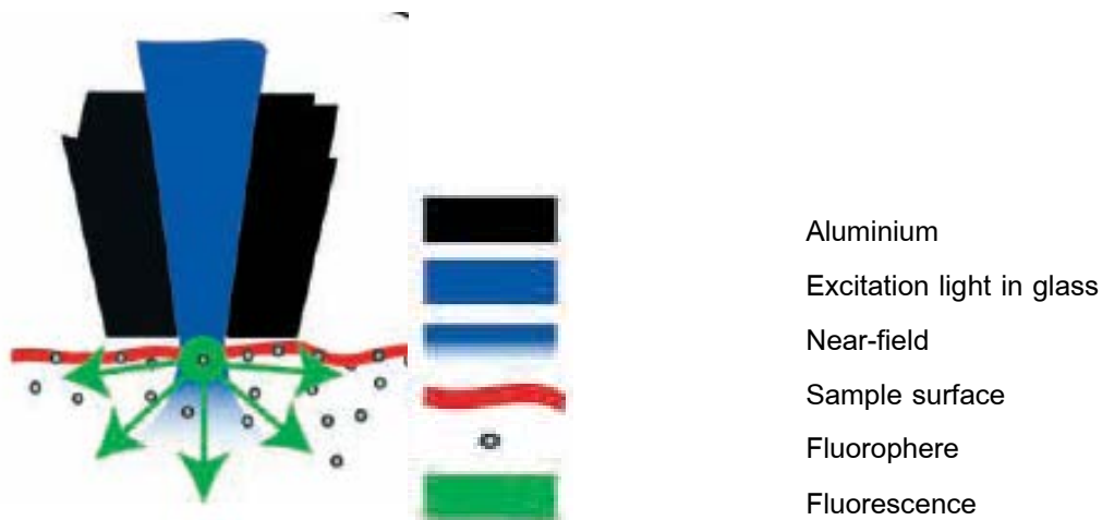
Figure9 The principle of surface-specific excitation. The optical near-field generated at the aperture has significant intensity only in a layer of <100 nm from the aperture; lower lying fluorophores are therefore not excited. Hence, background fluorescence is effectively suppressed. This forms the basis for the high optical detection sensitivity of this technique.(Lange et al. , 2001)
