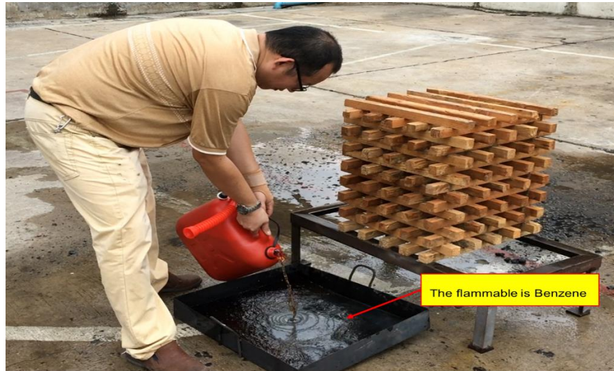
Figure 7 Preparing the burning area for testing fire extinguishers.
