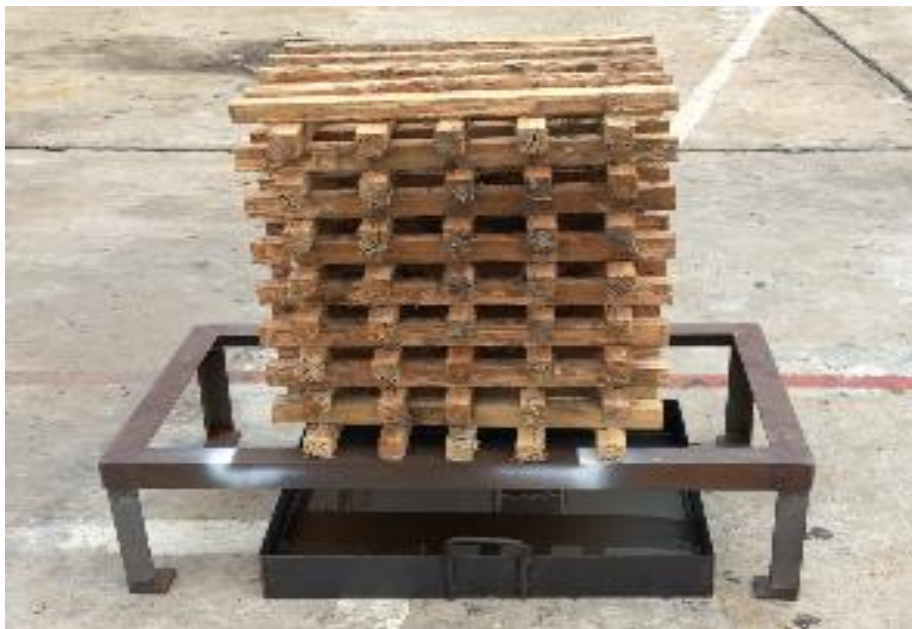
Figure 6 Preparing wooden curds for fire extinguishing rating test.
