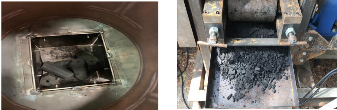
Figure 2 Coconut shell charcoal before and after reducing sizes with the double roller crusher
