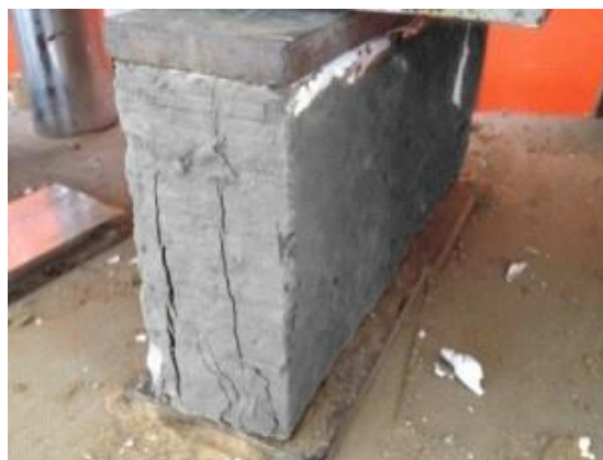
Figure 10 The failure characteristic of adobe bricks mixed with plastic in the compression test
