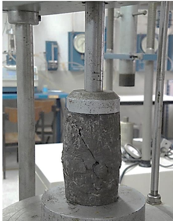
Figure 3 Failure characteristics of sample by the unconfined compression test
