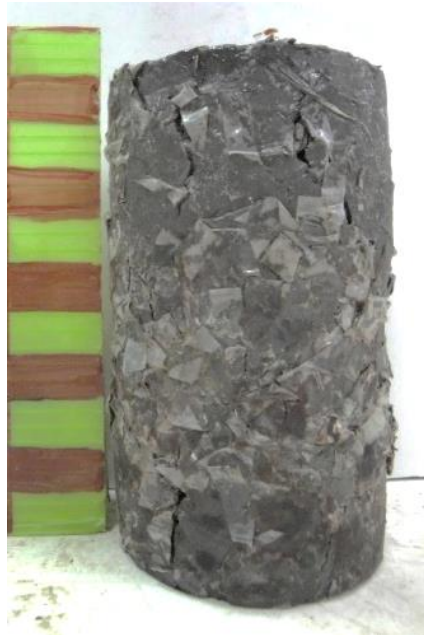
Figure 6 The characteristic of the mixed specimen with 2% amounts of plastic strips
