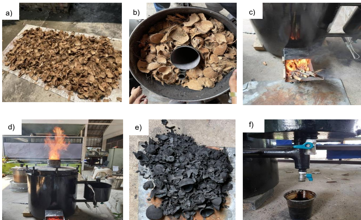
Figure 3 Charcoal production a) raw coconut shell, b) placing coconut shell inside carbonizer, c) igniting, d) carbonizing, e) charcoal and f) wood vinegar
