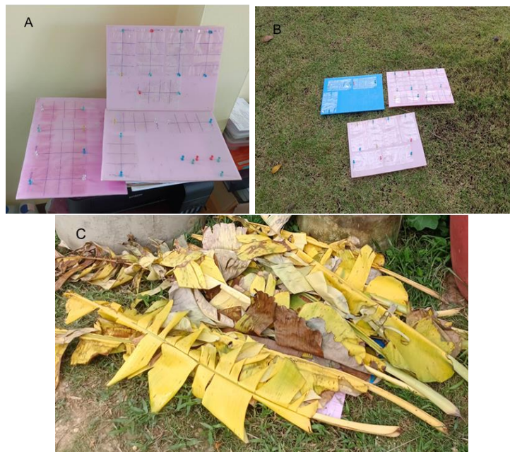
Figure 1 Samples exposed (A) indoor (B) outdoor (C) outdoor-hidden environments
